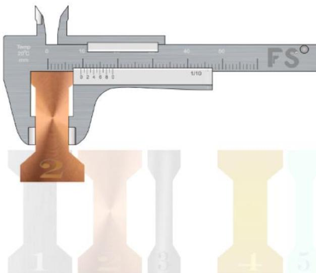
Figure 5. Callipers closed around sample to allow width to be measured.
