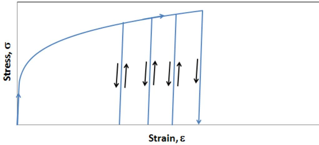
Figure 7. Strain cycling to work harden a sample.
