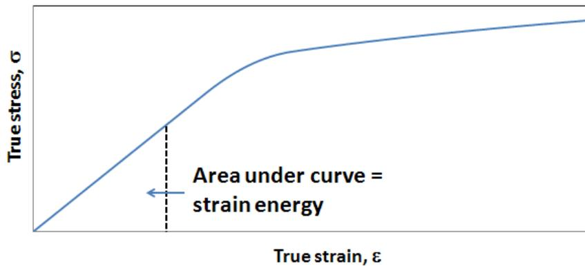
Figure 3. Calculation of strain energy from stress-strain plot.
