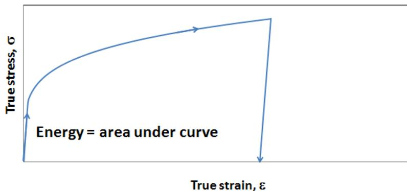
Figure 6. Calculation of work done (energy density) in tensile deformation.
