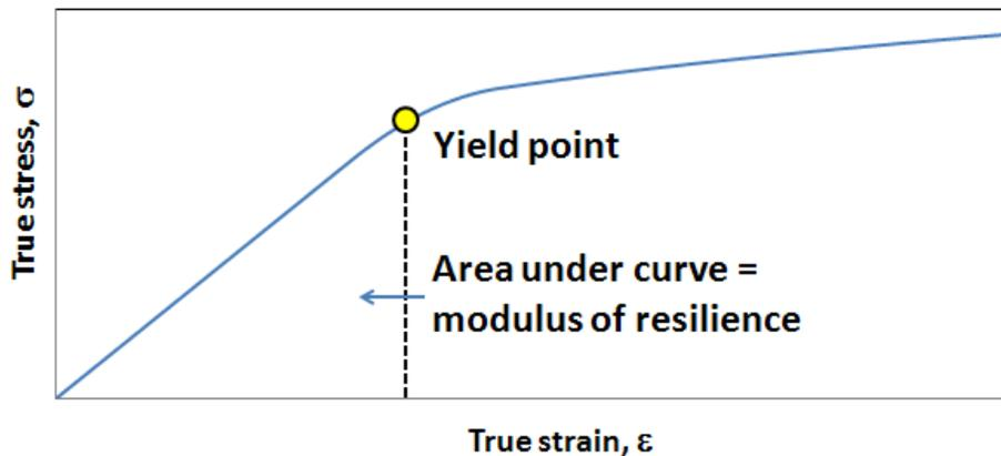
Figure 4. Calculation of modulus of resilience.
