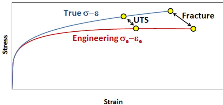
**Figure 2. True and engineering stress-strain curves for a material under tensile loading.**
