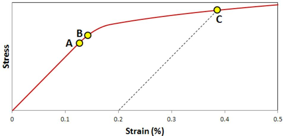
**Figure 1. Stress-strain curve of a material under low stress and key points labelled.**
