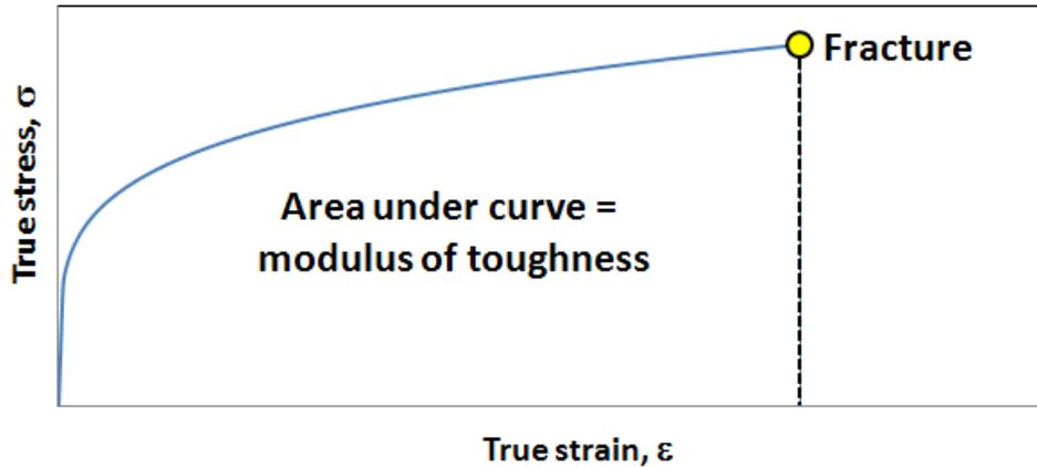
Figure 5. Calculation of modulus of toughness.
